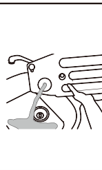
Drain the water out of water tank
